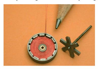
for easy manufacturing with conventional processes. Extending the system to two electrical phases, the generator can also be applied as a motor. It turned out that its power density can compete with available motors on the market. This talk will be presented at the 14<sup>th</sup> International Conference on Optimization of Electrical and Electronic Equipment (OPTIM 2014) in Brasov, Romania.
